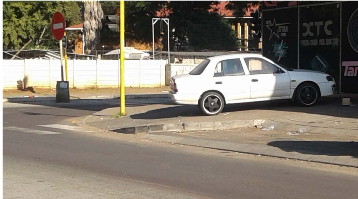
Figure 7: Bollards are largely installed to prevent vehicles from accessing and misusing pedestrian only areas. Bollards, and the installation thereof, are recommended but not listed as a technical requirement for NMT1 and, therefore, remain the prerogative of the designers/engineers or Municipality. If bollards are to be installed, it is recommended that they be installed according to the drawings in other parts of this NTR1 document
